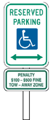
Required signage for standard accessible parking spaces
