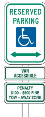
Required signage for van accessible parking spaces
